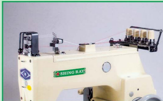
顶面中央给线系统与改良式给线装置。 Top center threading system and revised thread feeder.
